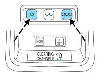
• After about 20 seconds, the message CHANNELS CLEARED will appear on the display. Do not hold for longer that 30 seconds. HomeLink® is now in the train (or learning) mode and can be programmed at any time beginning with step 2 in the "Programming" section.
